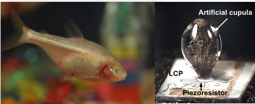
Biomimetic MEMS flow Sensors inspired by the superficial neuromasts in blind cavefish
