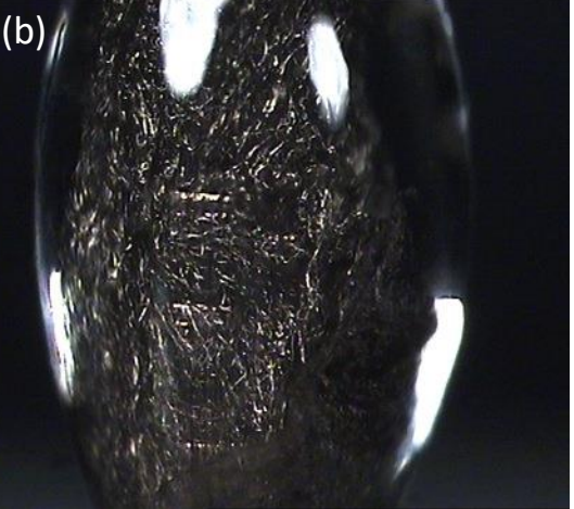
Microscopic images of (a) MEMS Artificial neuromast flow sensor (b) Zoom-in view showing the encapsulated cupular fibrils
