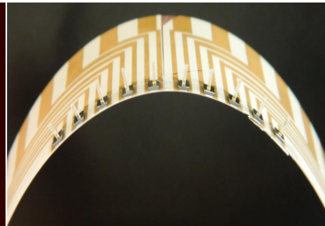
Array of 4 \times 5 of the piezoelectric sensors mounted on flexible LCP
