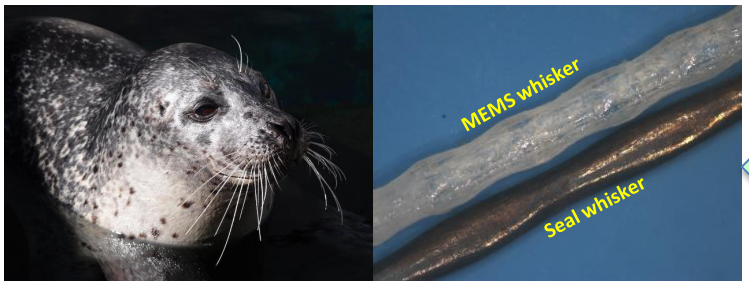
Harbor seal whisker inspired MEMS flow sensors to reduce vortex-induced vibrations
