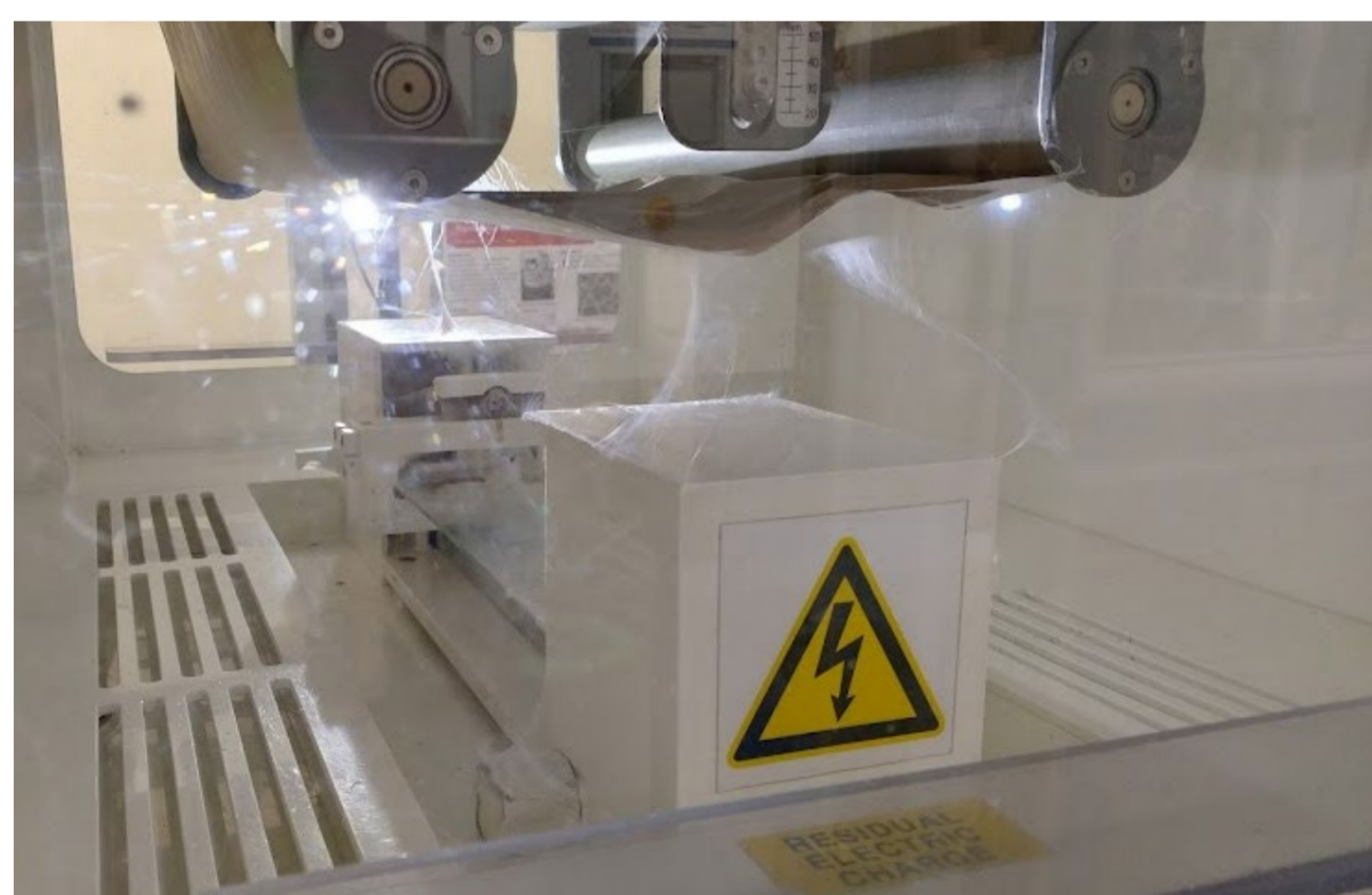
Figure 2: Preparation of the bipolar membranes with electrospinning. Left: picture of an electrospinning process. Right: schematic representation of the BPM fabrication steps.
